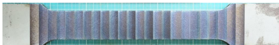
Fig.3 Laser-treated tensile test coupon.
